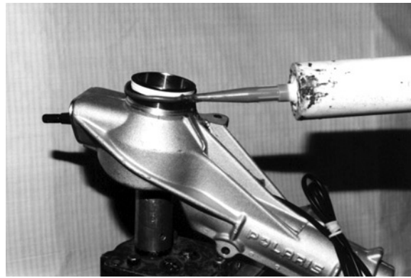
Loctite® 587™ Blue High Performance RTV Silicone Gasket Maker seals and retains the front wheel hub seal sleeve.
