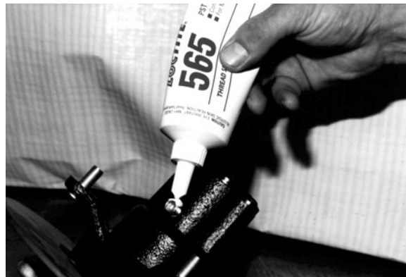
Loctite® 565™ PST® Thread Sealant is used on the magnetic drain plug found on the front wheel hub of all-wheel-drive model ATVs.
